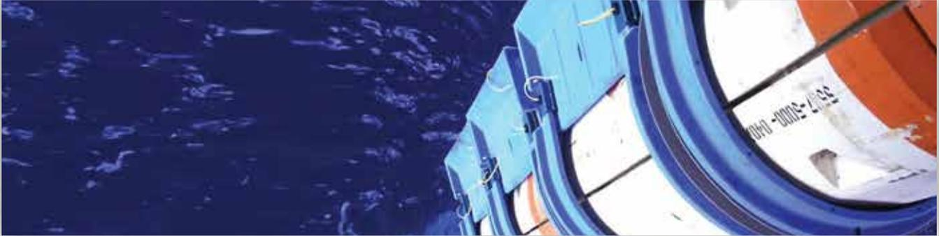
Tail Fairings™ provide excellent VIV suppression and drag reduction performance during deepwater drilling operations. These fairings streamline the flow of water around large-diameter tubulars and help minimize vortex shedding forces. In addition to reducing riser and wellhead fatigue, Tail Fairings also lower top and bottom angles in strong currents.
