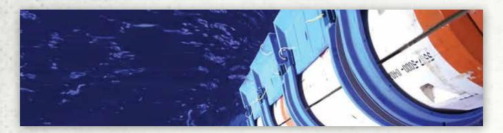
VIV Solutions' fairings provide excellent VIV suppression and drag reduction performance for deepwater drilling operations. Fairings work by streamlining the flow of water around large-diameter tubulars, thereby minimizing vortex shedding forces. In addition to reducing riser and wellhead fatigue, fairings also lower top and bottom angles in strong currents.
