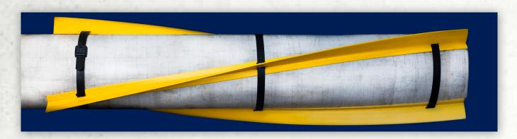
VortexVines<sup>™</sup> represent the next generation of helical strakes, a tried-and-true solution for suppressing vortex-induced vibration (VIV) of subsea tubulars such as risers, tendons, and pipelines. Helical strakes are also a popular choice for structures in wind such as industrial chimney stacks and even car antennas.
