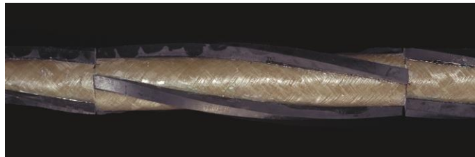
Figure 3 – Intentionally Misaligned Strakes
